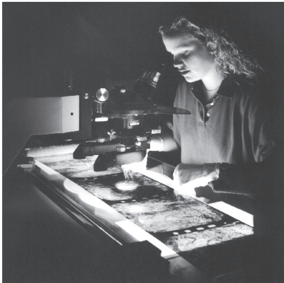
The library's top-ranked Map and Imagery Lab features sophisticated technology, such as this Z240 stereoscope, which aids in aerial photo interpretation.
